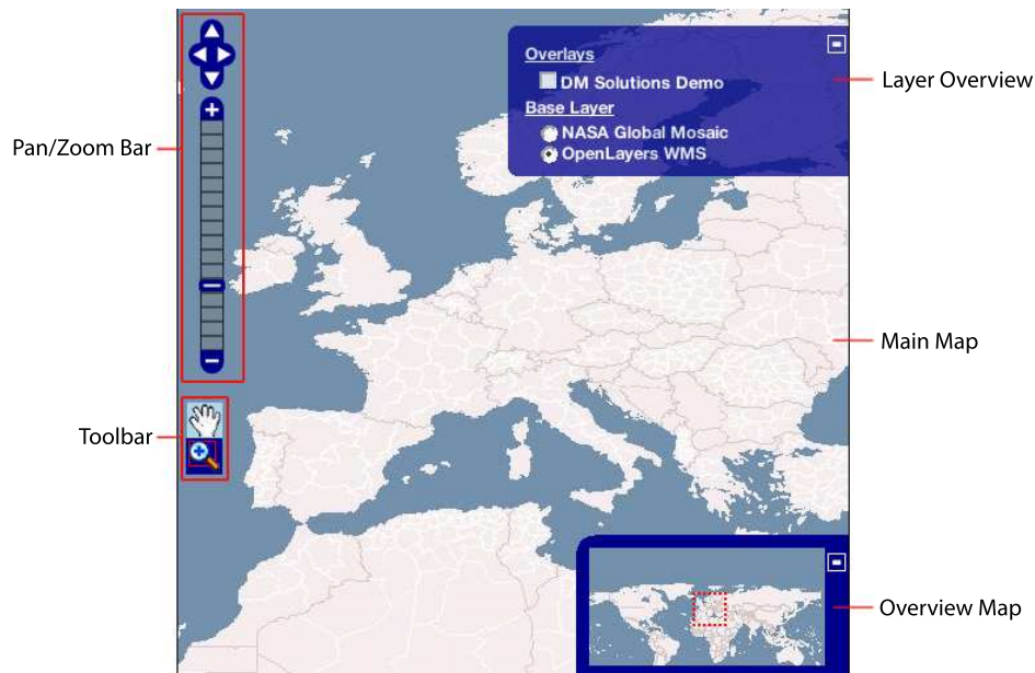
Figure 2.3: Components of Web Mapping Application OpenLayers
